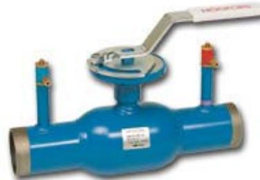
The Högfors V-port balancing valve is ideal for shut-off and control applications. The valve is supplied complete with upstream and downstream test points and an adjustable travel stop to set a balance position. If the valve is required to shut-off then full 90° operation can be achieved by simply removing a bolt, the bolt can be re-fitted without losing the preset balance position.
